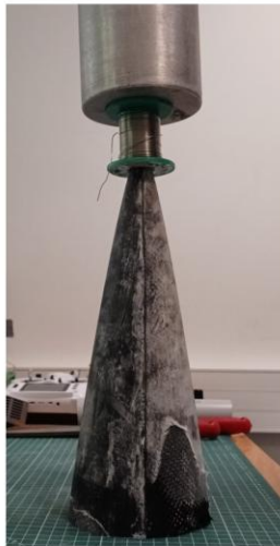
Figure 19: Compression test on the joined half parts of the nosecone.
