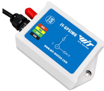
Figure 18 - module WTAHRS1 de Wit Motion
