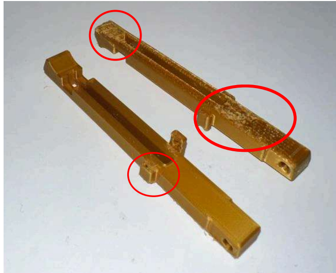
Fig 29: Unusable printed parts
