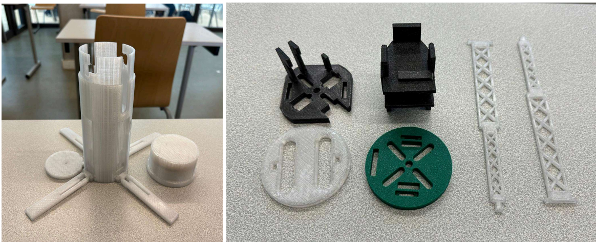
Fig 36: CanSat's PETG printed parts
