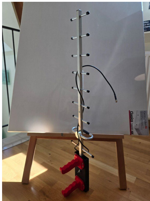
Figure 19 : Antenne YAGI 12 dB
