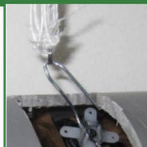
Figure 1 : Parachute release system.
