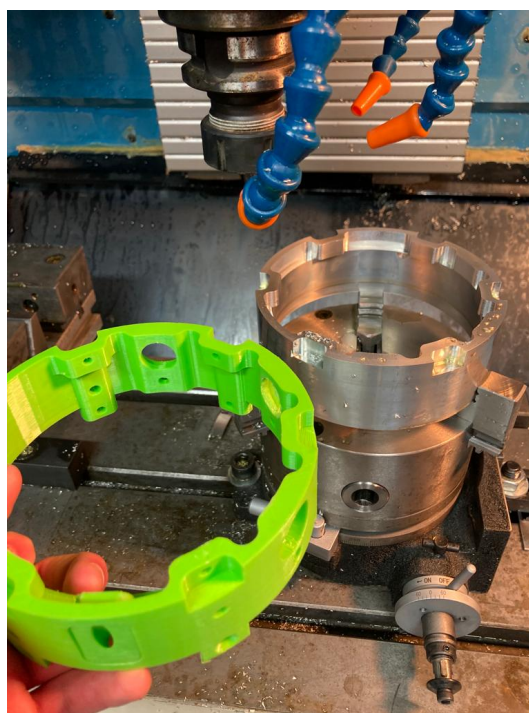
Figure 5: Usinage de la bague elec
