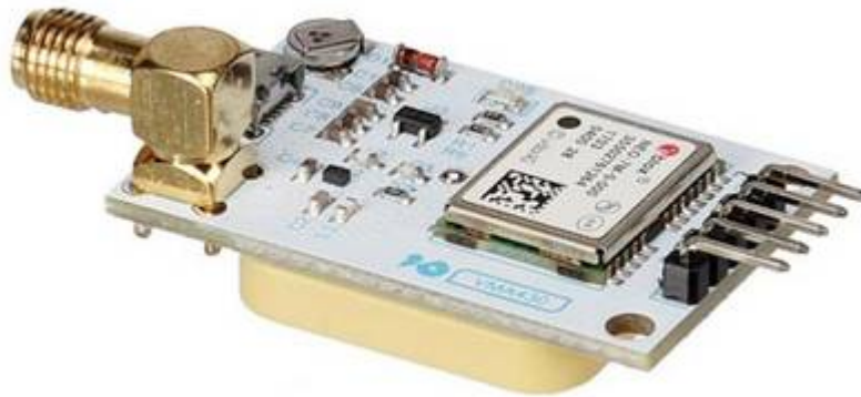
Module GPS U-Block Neo-7M WPI430
