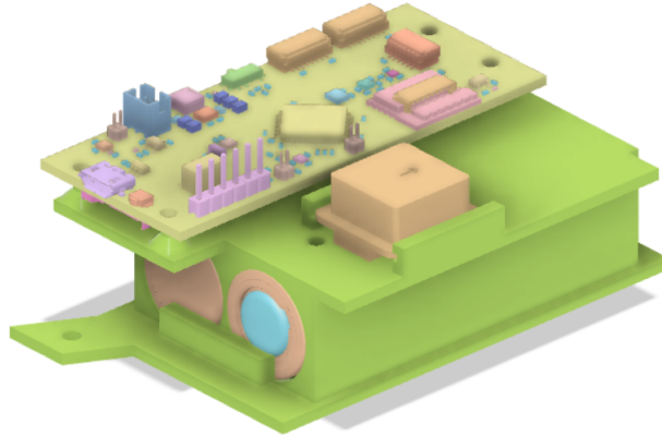
Figure 9: Support of the PCB, the battery and the GPS
