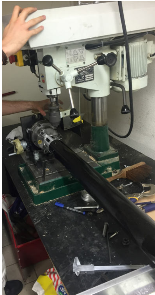
Figure 24: perçage du corps
