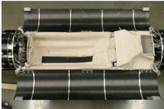
Fig. 3.5 Ejection system bay
