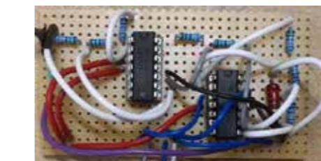
Finished amplification card – some wires are not connected yet.
