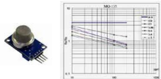
Fig. 3 MQ135 and sensibility characteristics
