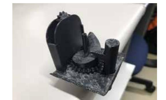
Fig. 2. Striking mechanism (prototype)
