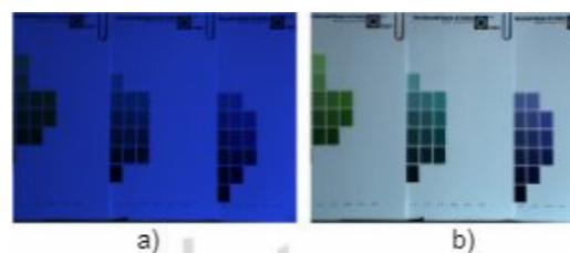
figura 14. a)original image b)Processed image with white patch algorithm.
