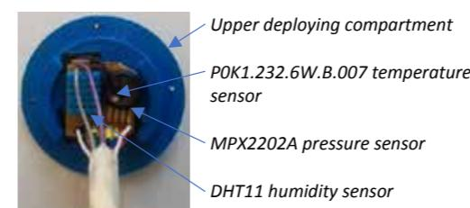
An amplification card is connected to the outputs of the sensors, so the measures can be sent to the core of the CanSat.
