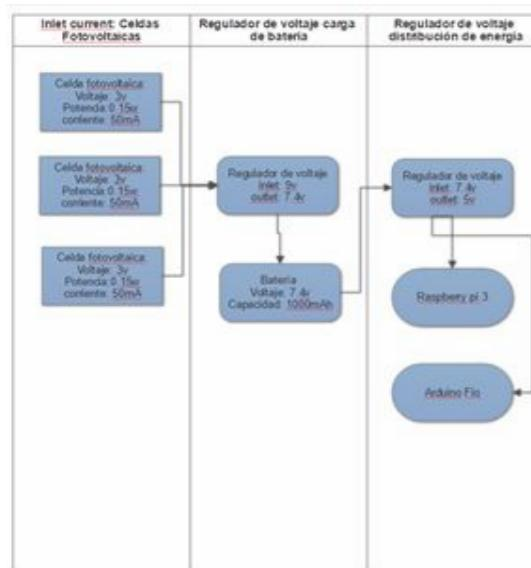
Figure 10. Diagram system power.
