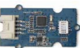
Fig.4 Multichannel Gas Sensor
