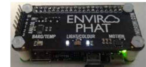
Core system – the ADC is on the left of the Enviro pHAT additional card, and the Raspberry Pi Zero is under it.
