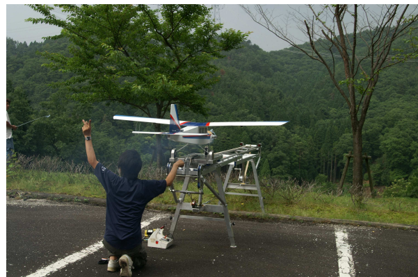
Fig. 5 Launch of Small UAV
