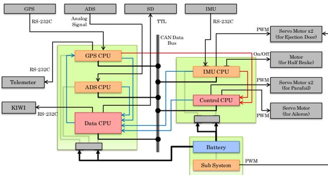
Fig. 11. Onboard avionics of Ninja-10.
