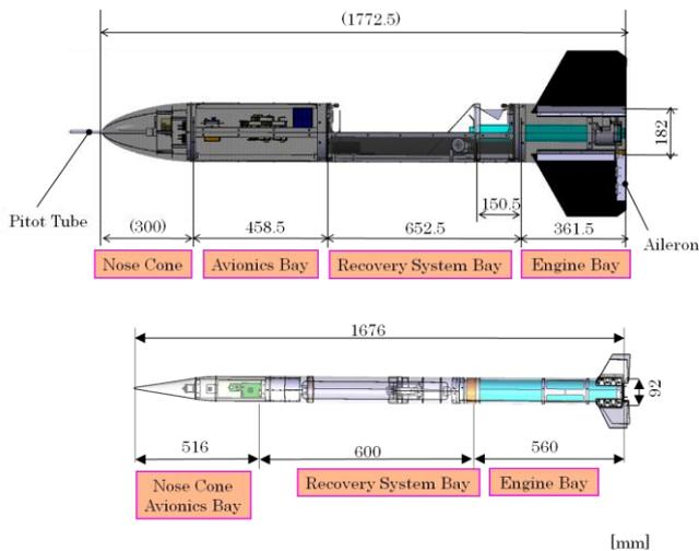
Fig. 3. KIT student's experimental rockets.
