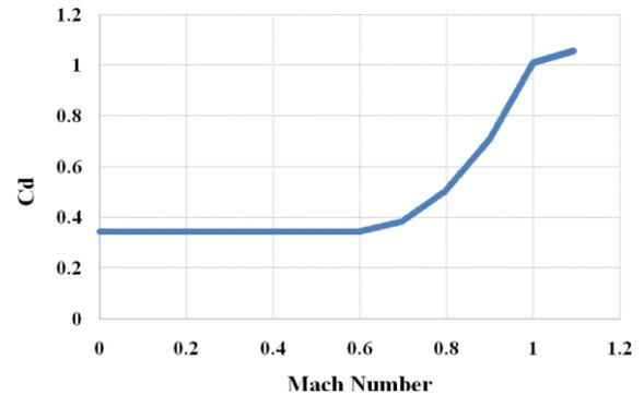
Fig. 4. Drag coefficient of Sakura.
