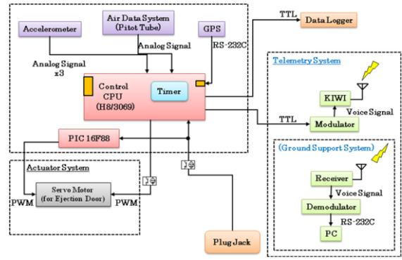
Fig. 12. Onboard avionics of Sakura.
