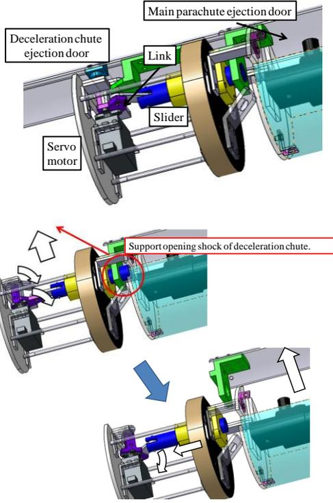
Fig. 10. Door ejection mechanism.
