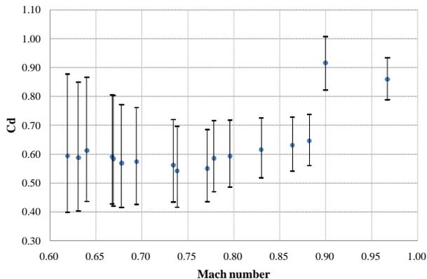
Fig. 21. Calculation of drag coefficient.
