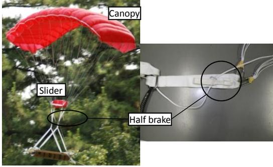
Fig. 5. Parafoil's canopy, slider, and half brake.
