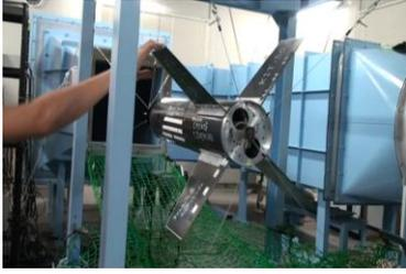
Fig. 14. Wind tunnel test to check aileron controllability.
