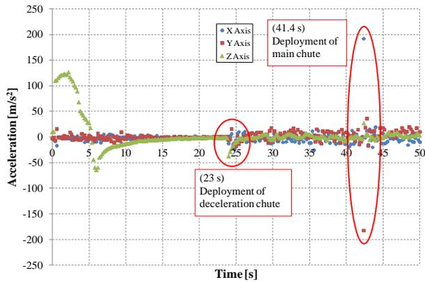
Fig. 19. 3-axis acceleration change.
