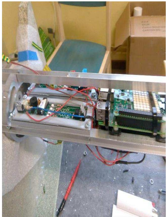
*Figure 2: Centrale inertielle*
