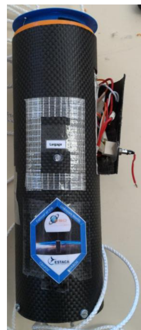
The CanSat during the final integration with windows to fit components, closed with Kevlar-reinforced tape.
