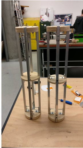
Figure 12: Structure prototypes with U and square profiles
