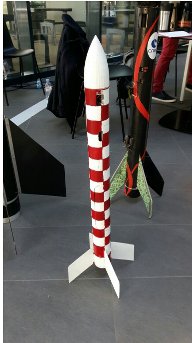
Figure 8: Panoramix mini rocket based on skin structure (built by some Solinas members in 2015/2016)
