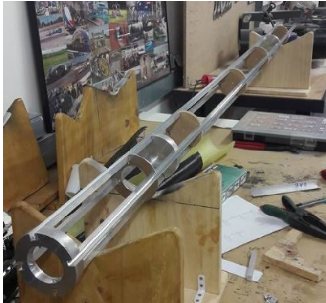
Figure 7: Solinas internal structure
