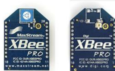
Fig.6 : On the left a XBEE with an antenna on chip and on the right a XBEE with an U.FL connector
