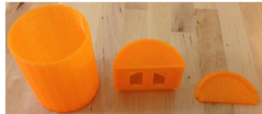
Fig. 9 The 3 parts of the can realised using 3D printing process
