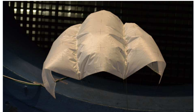
Fig.4. Stability and Piloting test in wind tunnel
