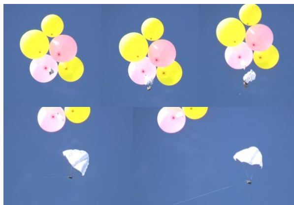
Fig. 4. Parachute deformation during an opening test
