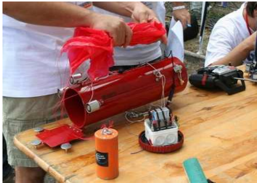
CanSats are installed in a PVC tube from which they drop when the door is opened
