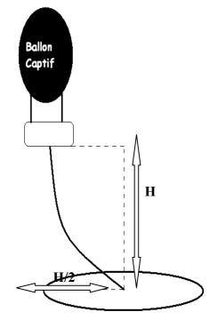
Note: The cansat released point can be moved by the organisation (by moving the attachment point on the ground), depending of weather conditions.
